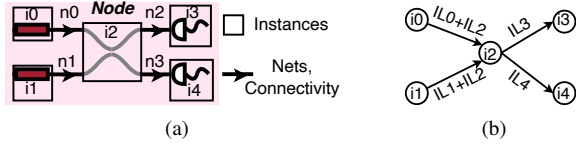
Fig. 2: (a) Node-level circuit topology definition and (b) corresponding weighted direct acyclic graph (DAG) representation.
